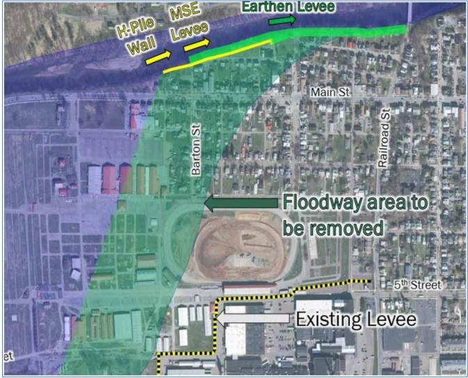
Figure 4.8 Depiction of Impacts on Floodway Resulting from Alternative A-3
