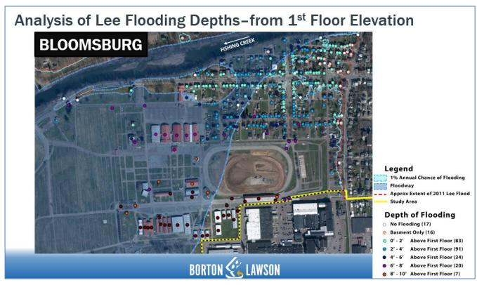
Figure 5.3 Modeled Depth of Flooding in Structures in West End of Bloomsburg from 2011 Flood Lee
