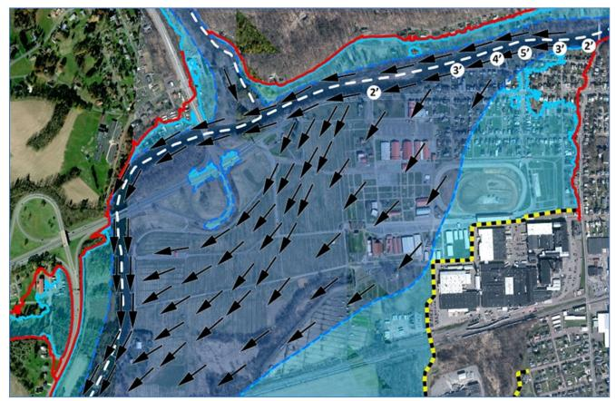
Figure 4.6 Flow Vectors of Fishing Creek and Floodway
