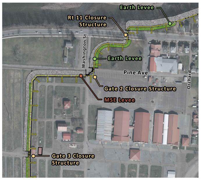
Figure 7.10 Proposed Levee Design from Route 11 Closure to Gate 3 Closure
