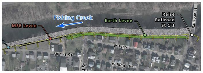
This reach of the line of protection is on an alignment with minimal lateral clearance through the residential area. The riverside levee slope will be protected by 18 to 24" riprap.
