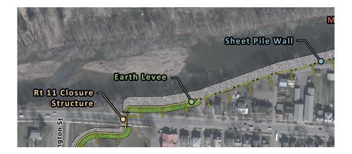
Beginning at Sta. 22+50, an earth levee will extend to the Route 11 road closure structure abutment at Sta. 25+70+\_. The stop log closure across route 11 is approximately 6 feet in height if the roadway is not raised. Being a state highway and also being in the floodplain, it was determined that the road should not be raised to lower the activation frequency.
