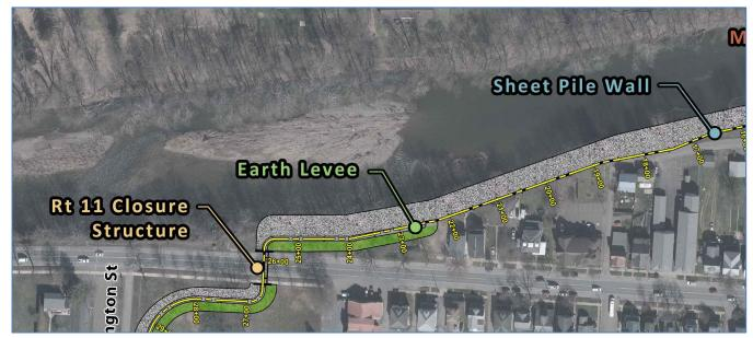
Figure 7.9 Proposed Levee Design Near Route 11 Closure Structure
