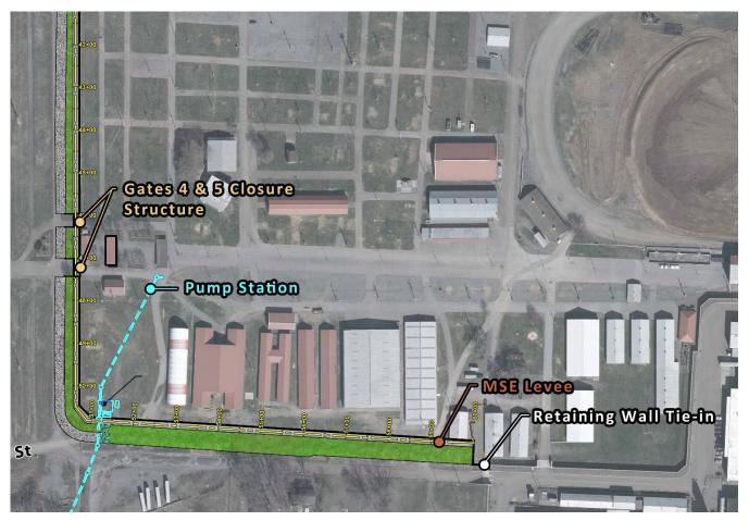
Figure 7.11 Proposed Levee Design from Gates 4 and 5 Closure to Tie-in Location
